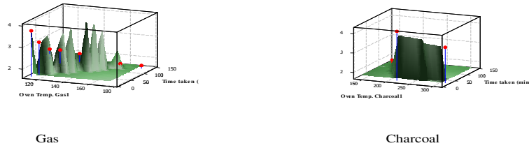
Fig. 4: Response of Fish Weights (kg) to Relationship between Kiln Temperatures (°C) and Time Taken (min) at D 1 ; (125 mm)
