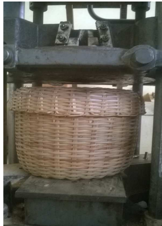
Universal Testing Machine (UTM) Figure 3: Basket subjected to compression test
