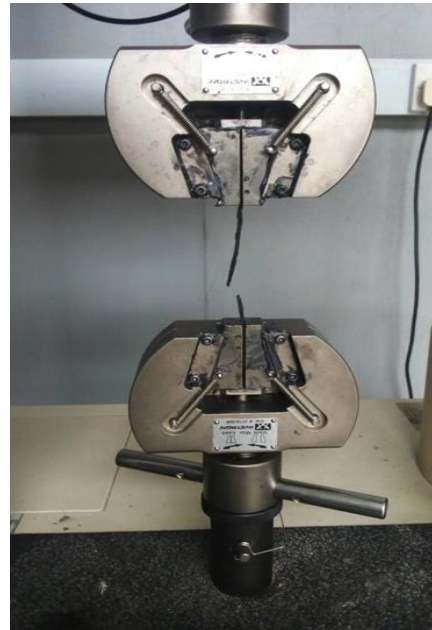
Plate 2: Tensile Test on Specimen
