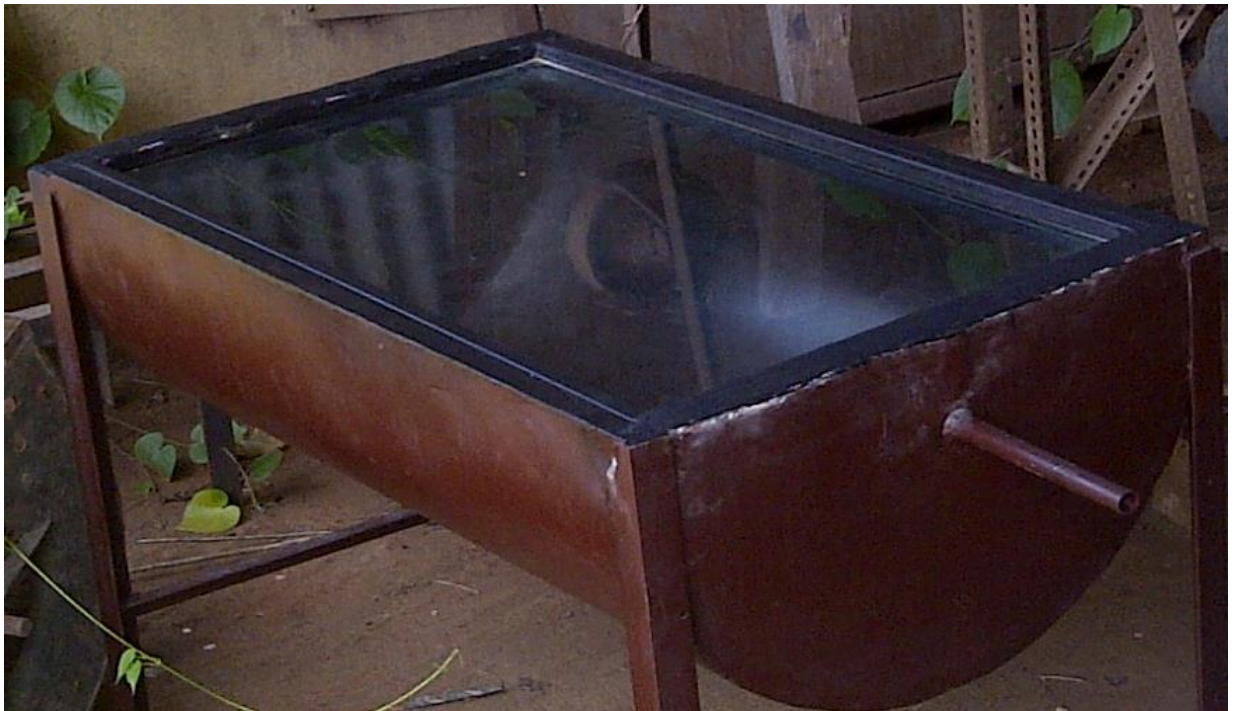
Figure 2: Thermal Storage Chamber
