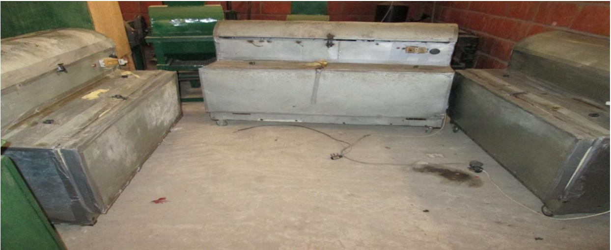
Plate1: Three cabinets of galvanized aluminium sheets for laboratory storage of onion bulbs.
