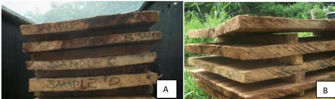
Fig.1: Wood stacked in the solar kiln (A) and wood stacked in open air environment (B)
