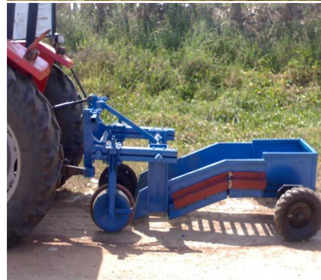
Picture of the improved harvester in trailed position for harvesting
