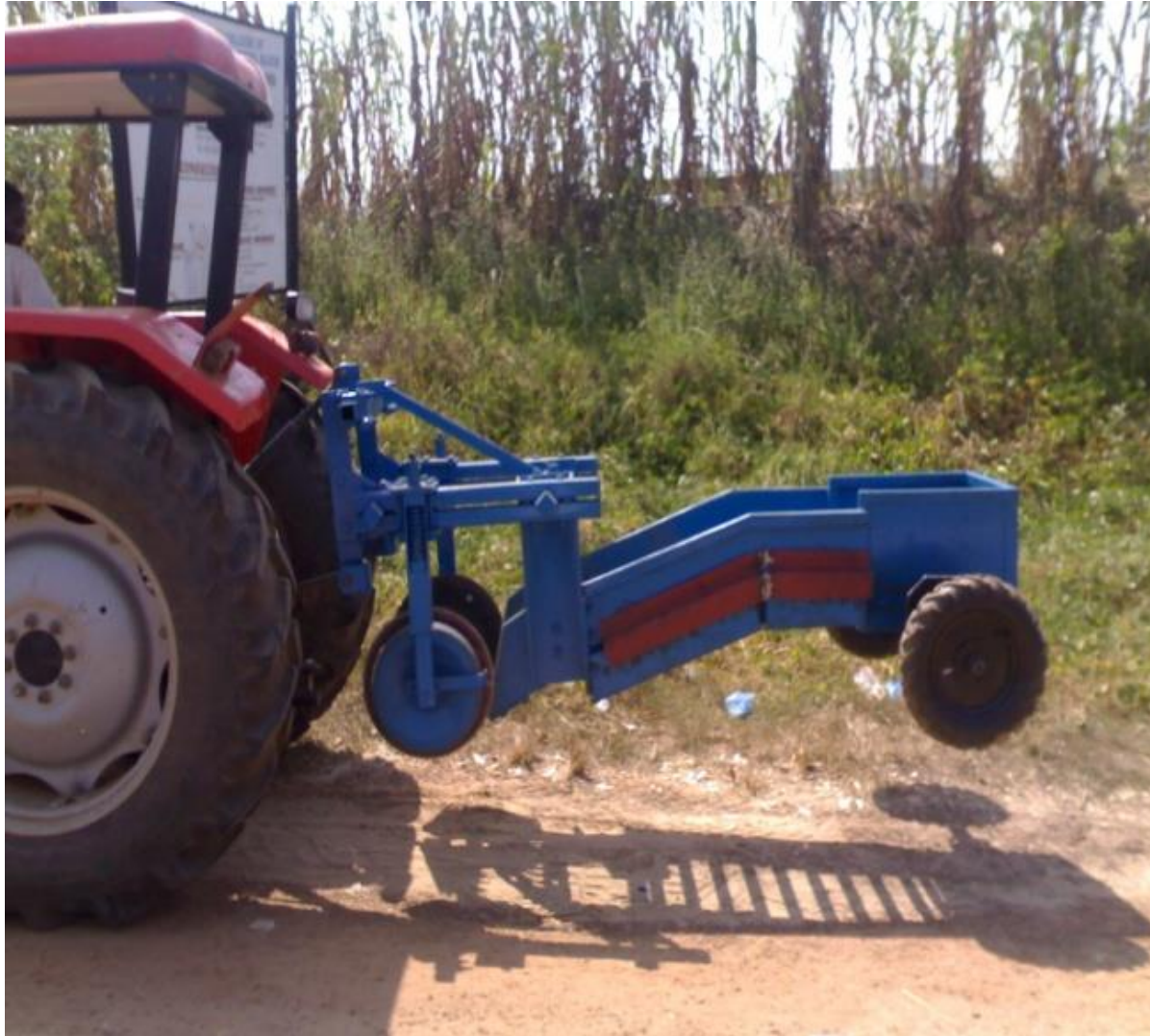
Picture of the improved harvester in transport position, lifted by the tractor
