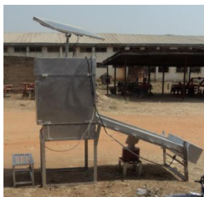
Plate I: Side View of the Hybrid Solar Dryer
