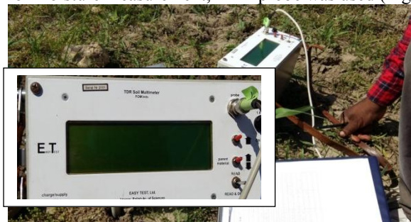
Fig.3. Soil Moisture Measurement with TDR probe Multimeter
