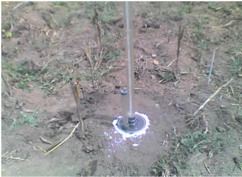
Figure 2. Disc permeameter on a zero Tillage plot
