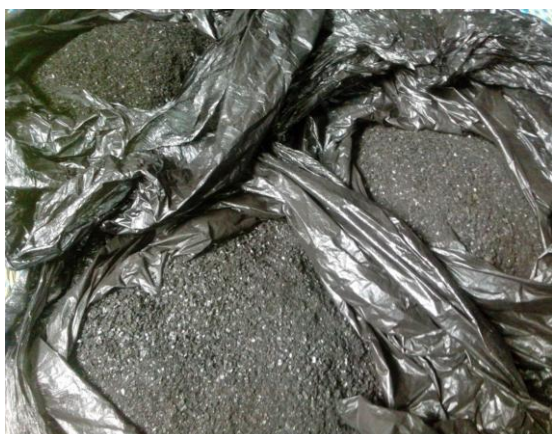
Plate 3: Experimentally Produced Granular Activated Carbons (GAC)
