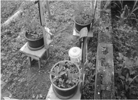
Plate 2: Lysimeter Setup for Lagos Spinach ( Celosia argentea ) Amaranth ( Amaranthus cruentus )
