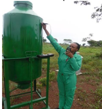
Figure 5: Temperature reading using therma probe for double walled insulated metallic silo
