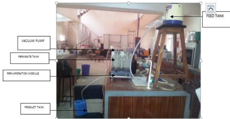
Figure 18: Set up of a pervaporation unit for bioethanol dehydration at the Dept. of Agricultural and Environmental Resources Engineering, University of Maiduguri, Maiduguri, Nigeria
