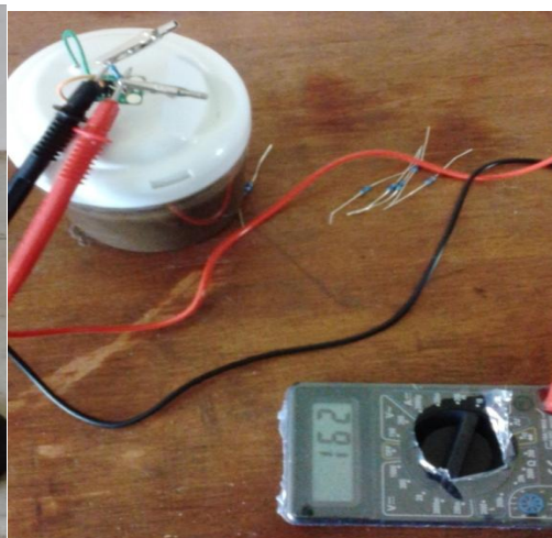
Plate 2: Multi-meter connected for voltage measurement
