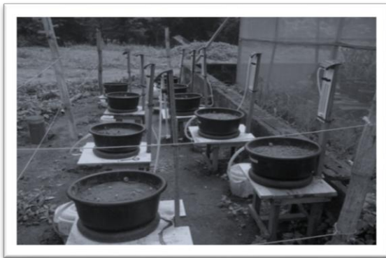
Plate 1: Typical Setup of the Weighing Type Lysimeter.
