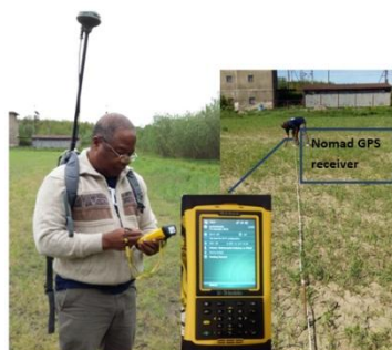
Fig.1. Marking out the Experimental Plot with Nomad/Trimble GPS Receiver
