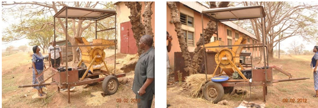
Fig. 9: Picture of solar- powered rice threshing machine at the University of Agriculture, Makurdi
