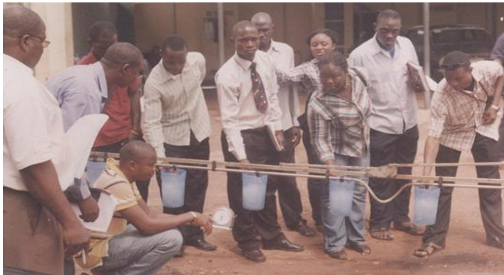
Figure 1: Static calibration method of boom sprayer at the Department of Agricultural and Bio-Environmental Engineering, Auchi Polytechnic, Auchi, Edo State, Nigeria.
