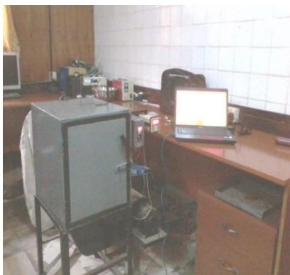
Figure 2.1: Dryer with Associate Instrumentation
