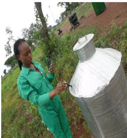
Figure 6: Temperature reading for single walled aluminium sheet silo
