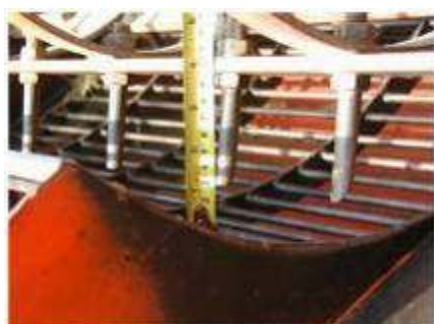
Figure 3: Setting the clearance peg-teeth and concave.
