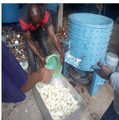
Plate 1 (a and b) Testing of Peeling Machine (a) and Grater (b)
