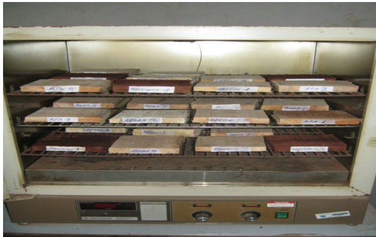
Figure 5: Experimental set up for moisture content determination by oven-dry method
