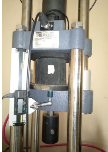
Figure 2. Test for the compressive strength of the briquette using a Universal Testing Machine
