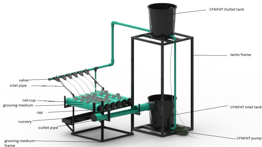
Figure 1. A 3-D View of the designed combined flow nutrient film hydroponics system
