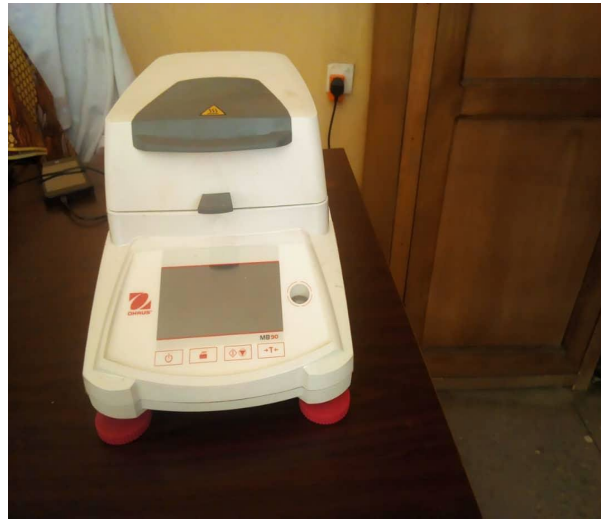
Figure 1: Pictorial View of the Instrumented Dryer Figure 2: Moisture Analyser (OHAUS MB 90)
