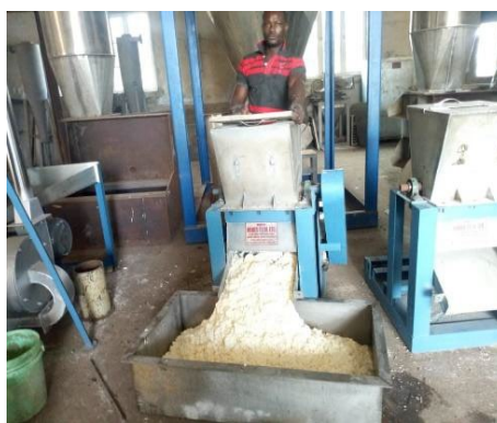
Plate 1 (a and b) Testing of Peeling Machine (a) and Grater (b)
