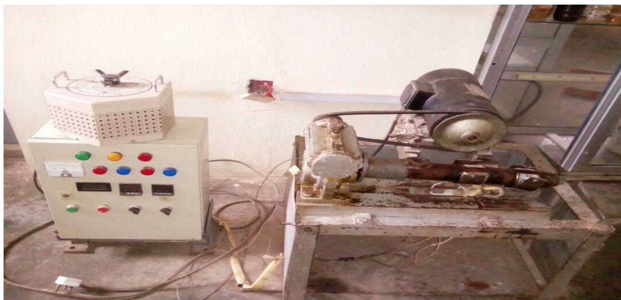
Plate 3: A laboratory model rotating screw extruder
