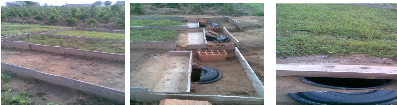
Fig. 1. (a) Layout of the plots, (b) Layout of the plots showing the collector and the collecting tank and (c) Picture of the Broad-leaf carpet grass
