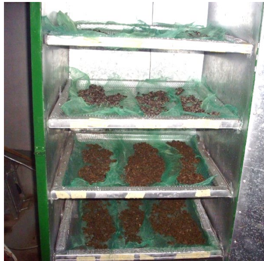
Figure 3. Arrangement of Locust beans in the Dryer
