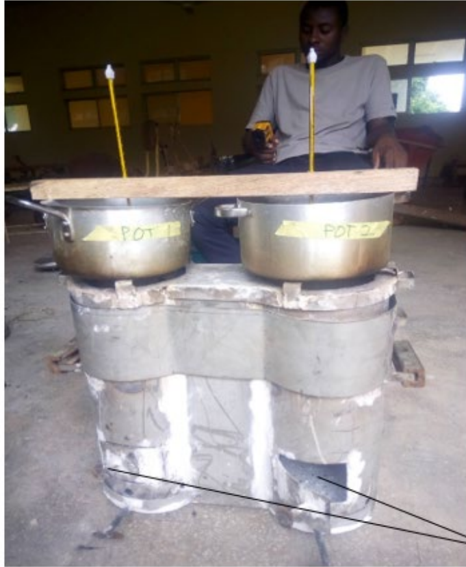
Plate 2.1: Experimental setup with pot 1 and 2 been operated on closed and moderately opened air vents, respectively
