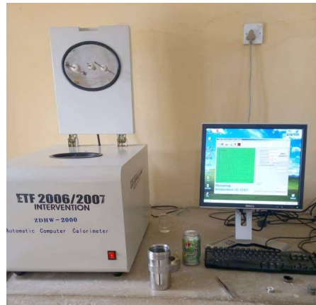
Figure 1. Test for the calorific value of the briquette using a bomb calorimeter
